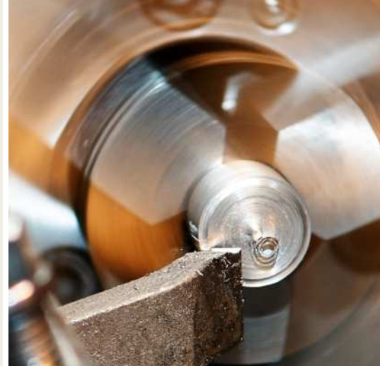
Counterbores for solderless tube connection (DIN 3854/DIN 3862)
