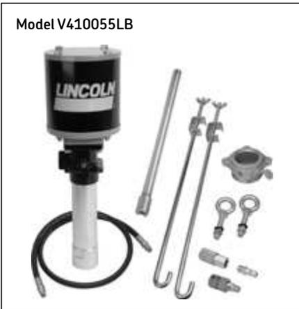
**Model V410055LB 10:1 55 gallon (208 liter) lubrication truck pump with bung bushing**
